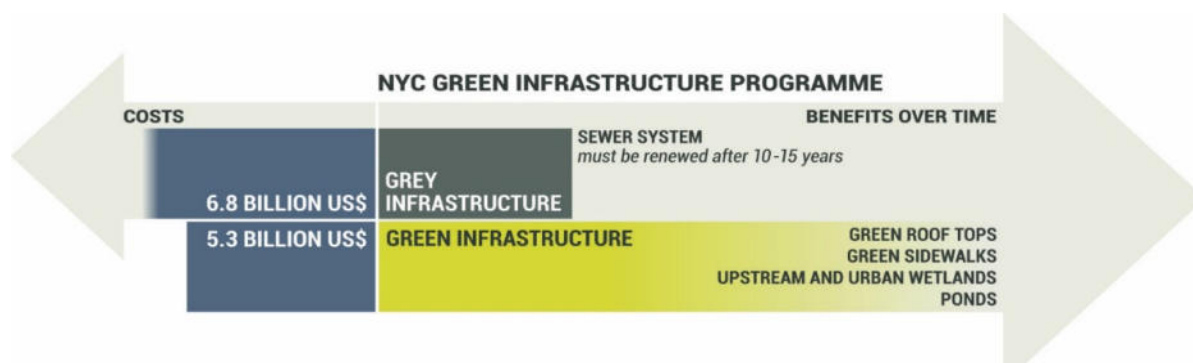
Figure 1. Green versus grey infrastructure cost-benefit analysis for New York City. Source: NYC, 2010
